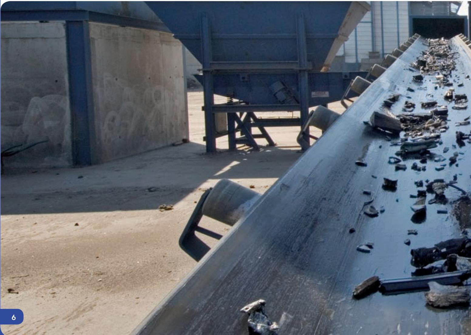
Steel cords **reinforce resistance** to longitudinal slitting that may be caused by foreign bodies or by the transported product itself.
